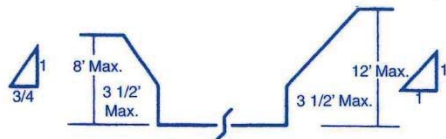
UNSUPPORTED VERTICALLY SIDED LOWER PORTION
